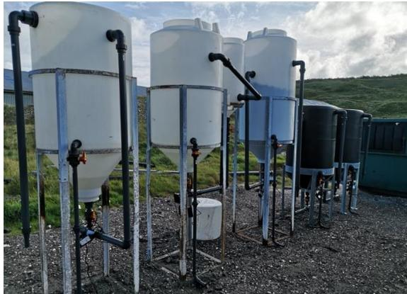
**FIGURE 2. PILOT-SCALE ACTIVATED SLUDGE SET-UP AT A COMMERCIAL MARINE RAS. COURTESY: CARLOS OCTAVIO LETELIER**
