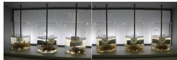
**FIGURE 1. SCREENING OF FLOCCULENT CHEMICALS WITH JAR TESTS. COURTESY: JOUNI VIELMA**
