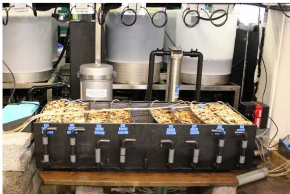
**FIGURE 2. EXPERIMENTAL WOODCHIP BIOREACTOR SET-UP IN LAUKAA, FINLAND. COURTESY: JANNI PULKINEN**
