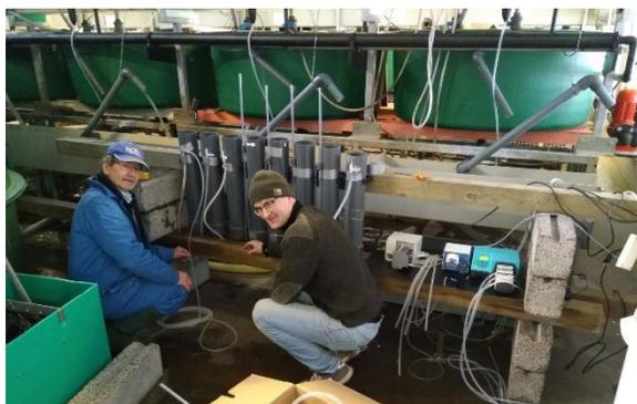
**FIGURE 4. EXPERIMENTAL SET-UP INVESTIGATING REACTIVE FILTER MEDIA FOR P REMOVAL.**
