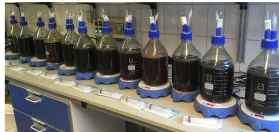
FIGURE 1. EXPERIMENTAL SET-UP TO INVESTIGATE THE HYDROLYSIS PROCESS AT DIFFERENT SALINITIES.
